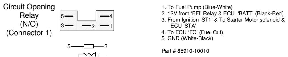
N.B. Diagrams are of relay plugs as viewed from above fuse box, not underside of actual relays
