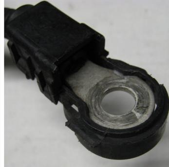
Single black wire (heavy gauge) – connected directly to Battery
